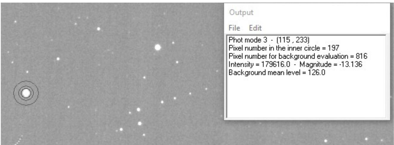
The software has the feature to place an aperture with 3 circles around the target star<sup>2</sup>. The inner radius  $r_1$  is so big, that the inner measuring circle contains all the light from the star<sup>3</sup>. The outer ring (between  $r_2$  and  $r_3$ ) measures the background mean level. In this case the background from the city and the moon is 126 ADU/pixel.
