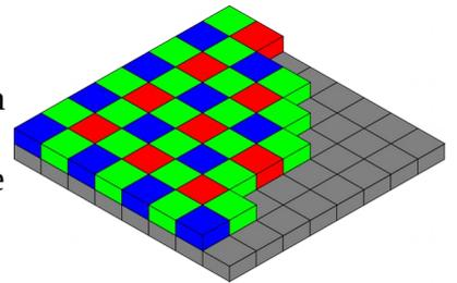
One of the main facilities of this sensor-type is the simultaneous observation of the star through four filters. It is especially interesting, that the two green layers gives two independent observations of the same star. The difference  $G2 - G1$  is a fine measure of how accurate the star is observed.
